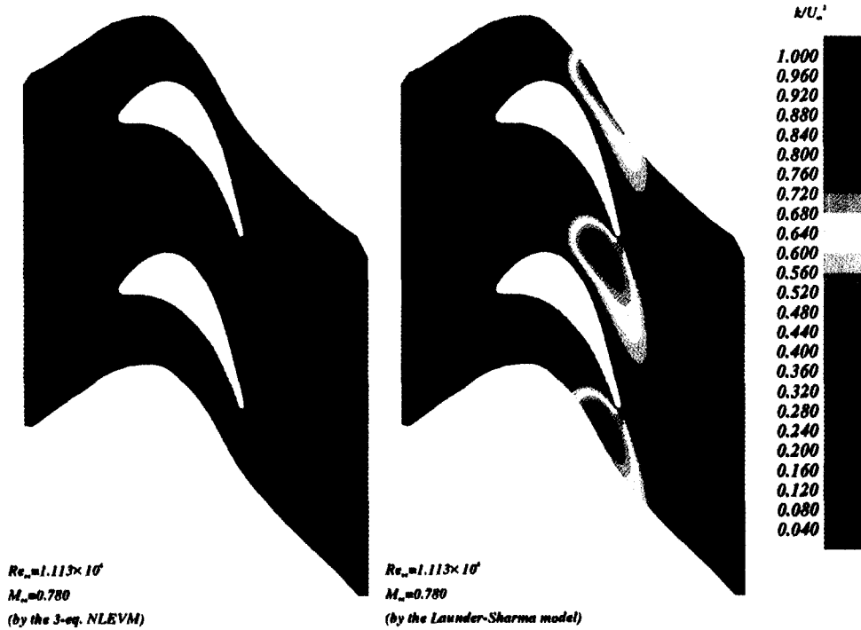
Figure 17 Levels of turbulent kinetic energy through cascade: a) present N-LEVM predictions; b) L-S EVM predictions
